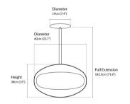
Cocoon Fires Aeris Burning Time: Up to 5hrs kW Output: 3.0 kW Features: • 360° Rotation • Converts to Pedestal
