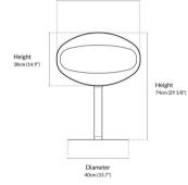
Cocoon Fires Pedestal Burning Time: Up to 5hrs kW Output: 3.0 kW Features: • Converts to Aeris
